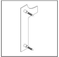
5. Screw the threaded rods into the back of the number/letter.
