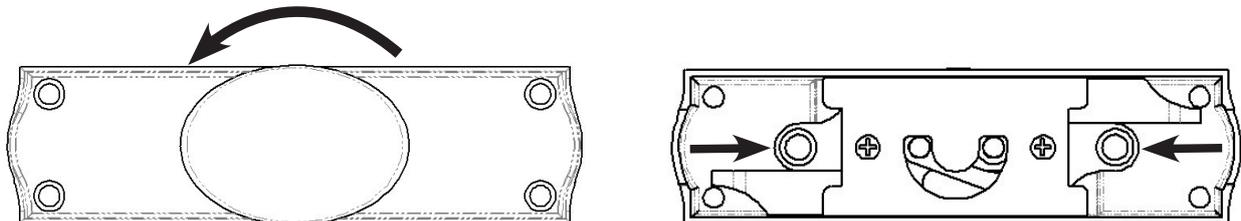
3. Connect one bolt to the mechanism by positioning one of the pins on the rear of the centre module into the 6.25mm hole in the bolt, measure the length you require this bolt to be, remove and cut to length, repeat this procedure for the other bolt.
