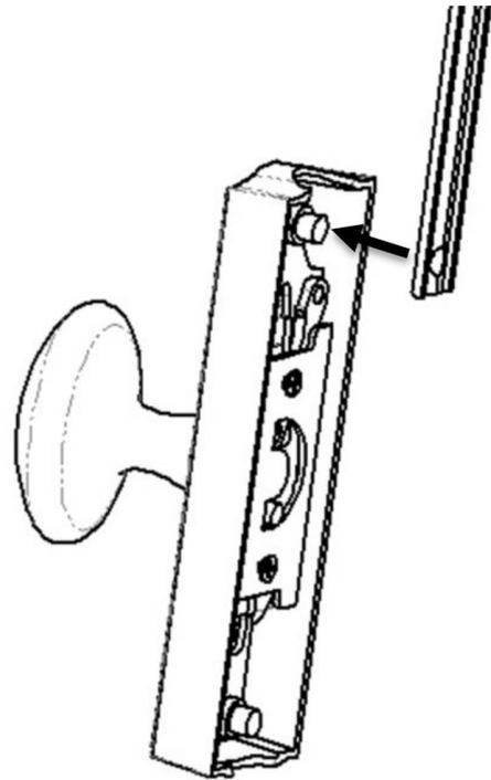
4. Once you have done this, fix the centre module to the selected position on your door using the 38mm long screws but do not drive screws fully as you need to be able to connect the bolts to the back of the mechanism.
