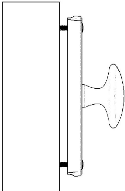
5. Maneuver the one of the bolts into the either of oval shaped holes in the centre module with the flat side to the door face, and connect the 6.25mm hole in the bolt to the pin on the back of the centre module mechanism.
