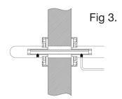
Check against the door to make sure that the length of spindle will fit through the door and locate with the opposite lever . "If fitting levers to doors thicker than 44mm A longer 120mm spindle (ALS1002H) will be required ."
