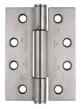
Grade 14 Concealed Bearing Triple Knuckle Hinge. Square (Max Load 160kg) They have a CE mark and are Certifire tested. BS EN 1935 rated. Comes with a 25 year mechanical guarantee and are fire door rated.
