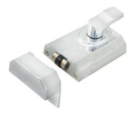
Contract Rim Cylinder Rollerbolt. 60mm. The standard latch has been replaced by a roller bolt which is sprung to allow the door to open and close on a simple pull or push and does not require the key or handle to operate in this position. Ideal for an external door application that has a pull handle only.
