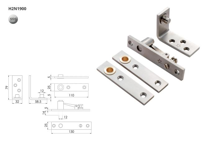
Standard Thrust Bearing Pivot Set (Max Load 80kg) Square or Radius options. Double Action Pivot Set which allows the door to be opened outwards in the case of an emergency. To be used in Conjunction with H2N1950 Emergency Release Door Stop. Comes with a 10 year mechanical guarantee.
