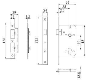
Contract Din Euro Profile Sashlock, 55mm. Square or Radius option. The Latch bolt has the Easi-T reverse function to save undoing the case so it can be reversed in seconds. Certified to BS EN 12209.
