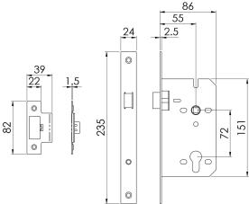
Contract Din Euro Profile Nightlatch. 55mm. Square or Radius option. The Latch bolt has the Easi-T reverse function to save undoing the case so it can be reversed in seconds.
