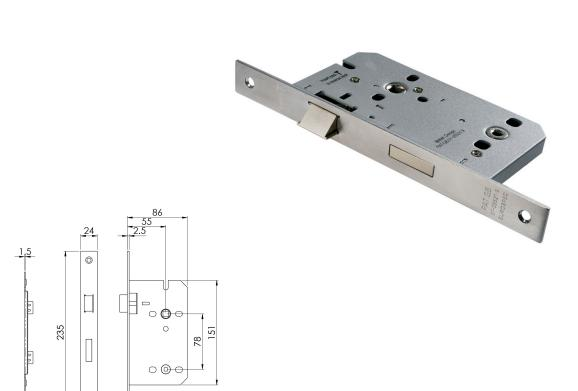
Contract Din Bathroom Lock 55mm. Square and Radius options. The Latch bolt has the Easi-T reverse function to save undoing the case so it can be reversed in seconds. Certified to BS EN 12209.
