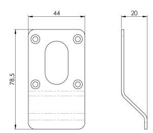
The Steelworx range of stainless steel cylinder pulls offers a wide selection of different profiles to choose from. Available in, Euro, Oval, Lock and Rim version and a Blank option. Fire door rated.
