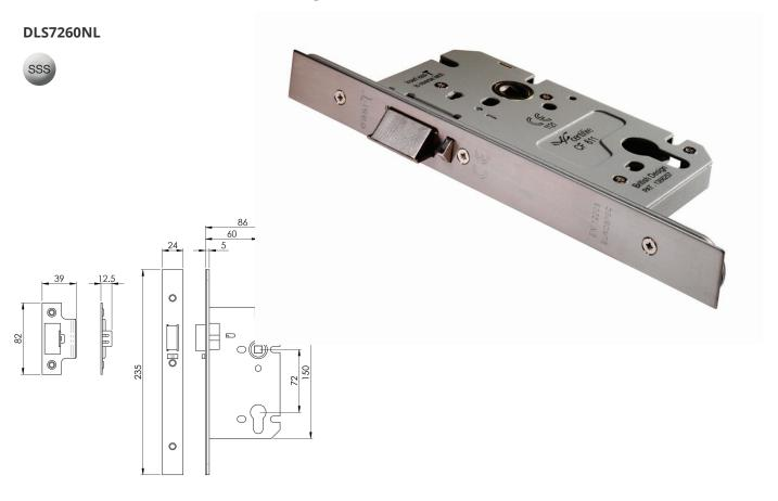
Easi-T Din Euro Profile Night latch 60mm. Square and Radius options. The Latch bolt has the Easi-T reverse function to save undoing the case so it can be reversed in seconds. British Standard BS EN 12209 and 179 Rated Sash lock used as a matter of course by the national house builders.
