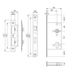
Easi-T Din Euro Profile Sashlock 60mm. Square and Radius options. The Latch bolt has the Easi-T reverse function to save undoing the case so it can be reversed in seconds. British Standard BS EN 12209 and 179 Rated Sash lock used as a matter of course by the national house builders.
