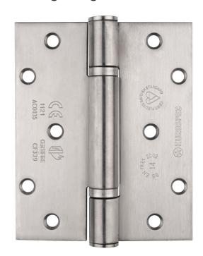
Grade 14 Thrust Bearing Hinge, Square (Max Load 160kg) Non removable pin. These are usually specified in heavy use commercial developments such as schools, hospitals, airports, public buildings. They carry a CE mark and are Certifire tested. BS EN 1935 rated.
