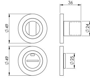
Designer Turn and Release without Indicator. Concealed fix screw on rose. Stylish bathroom turn & release, thumbturn on one side and an emergency release slot on the other. Part of the Steelwork range in Grade 316 Stainless Steel and will match all of the Steelworx levers.
