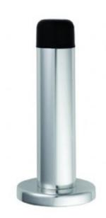
Cylindrical door stop with rubber buffer on a round rose. The base rose unscrews allowing it to be fixed to the wall or skirting board. The door stop main body is then screwed back on for neat concealed fix. Screw supplied.
