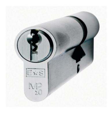
Euro Double Cylinder. These MP10 restricted 10 pin cylinders provide a high degree of security, having met the standards identified by Secured by Design the UK policed flagship initiative. Features include; anti drill, anti pick, anti bump, fire door rated. Keyed alike or master keyed options available.
