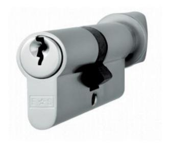
Offset Euro Cylinder and Turn. To lock the door on the inside, simply use the turn knob, there's no need for a key. These MP5 Architectural 5 pin cylinders provide a good degree of security. Fire Door rated.
