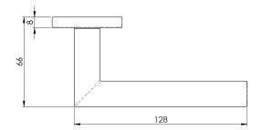
Lever on concealed fix press on round rose. Straight round bar lever neatly mitred where it adjoins the stem. Part of the Steelworx range in grade 304 Stainless Steel. Comes with a 10 year mechanical guarantee and is Fire Door Rated.
