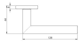
Lever on concealed fix press on round rose. Straight round bar lever neatly mitred where it adjoins the stem. Part of the Steelworx range in grade 304 Stainless Steel. Comes with a 10 year mechanical guarantee and is Fire Door Rated.
