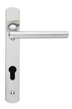
A straight round bar lever on a narrow backplate. It has a Euro profile keyhole 92mm c/c and operates a multipoint lock. Certified to BS EN 1906. Part of the Steelworx range in Grade 316 Stainless Steel.
