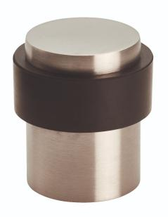
Flat top cylindrical door stop with a substantial rubber buffer circumference to protect doors. Concealed fixing. The lower section is screwed into the floor and the top is threaded into the base. Part of the Steelworx Stainless Steel range.
