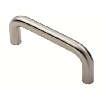
A robust and functional 19mm Dia. round bar D type pull handle, part of the Steelworx range in grade304 Stainless Steel, so ideal for internal and external homes and offices. Available in different sizes. These pull handles are fixed with 2no M8 threaded bolts through the door giving the strongest fixing possible.
