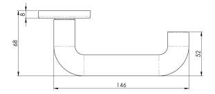
Lever on concealed fix press on rose. A substantial 22mm round bar return to door safety lever. Ideal for public/office doors where a more ergonomic operation is a necessary requirement. Part of the Steelworx range in grade 304 Stainless Steel.
