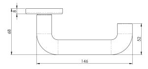
Lever on concealed fix press on rose. A substantial 22mm round bar return to door safety lever. Ideal for public/office doors where a more ergonomic operation is a necessary requirement. Part of the Steelworx range in grade 304 Stainless Steel.
