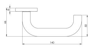
Safety Lever round bar return to door lever on concealed fix press on round rose. Lever available in 19mm or 22mm Diameter. Ideal for public/office doors where a more ergonomic operation is a necessary requirement. Part of the Steelworx range in grade 304 Stainless Steel.
