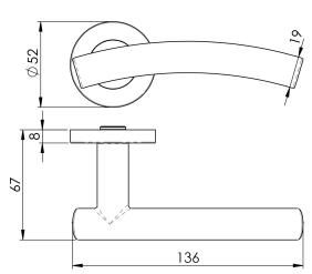
Lever on concealed fix press on round rose, Curved round bar lever (19mm) with a slightly higher than standard arch making it very ergonomic. Part of the Steelworx range in Stainless Steel. Comes with a 10 year mechanical guarantee and is Fire Door Rated. Suitable for domestic and commercial use.
