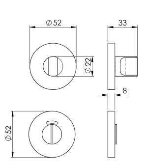
Standard Turn and Release with a vacant/engaged Indicator. Concealed fix press on rose. Stylish bathroom turn and release, thumb turn on one side and an emergency release slot on the other. Part of the Steelwork range in Grade 304 Stainless Steel and will match all of the Steelworx levers.
