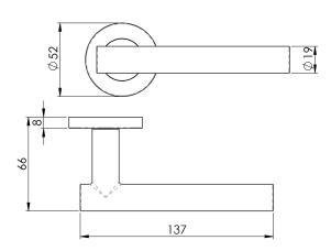
Lever on concealed fix press on round rose. A straight round bar lever neatly mitred where it adjoins the stem. Part of the Steelworx range in grade 304 Stainless Steel. Certified to BS EN 1906.
