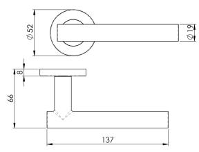
Lever on concealed fix press on round rose. A plain straight round bar lever sitting atop the stem. Part of the Steelworx range in grade 304 Stainless Steel. Comes with a 10 year mechanical guarantee and is fire door rated.
