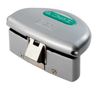
Push Pad Latch for use with panic exit devices. Fire door rated and comes with a 10 year mechanical guarantee. Certified to BS EN 179. CE mark and Certifire tested.
