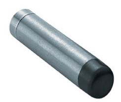
Cylindrical door stop with rubber buffer. The base rose unscrews allowing it to be fixed to the wall or skirting board. The door stop main body is then screwed back on for neat concealed fix. Screw supplied.
