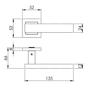
A square cut rectangular shaped straight bar lever on a concealed fix square press on rose. The mass of the handle faces forwards. An unfussy design which will blend well in a variety of applications. Part of a square themed designer lever collection in the Steelworx range in grade 304 Stainless Steel.
