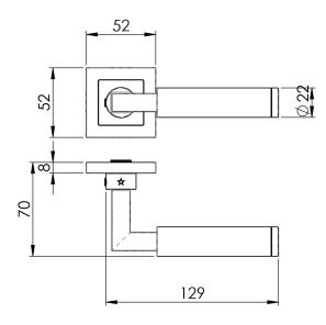
A square cut mitred lever extending into a smooth round bar on a concealed fix square press on rose. Part of a square themed designer lever collection in the Steelworx range in grade 304 Stainless Steel. Certified to BS EN 1906 standard and is fire door rated. Comes with a 10-year mechanical guarantee.
