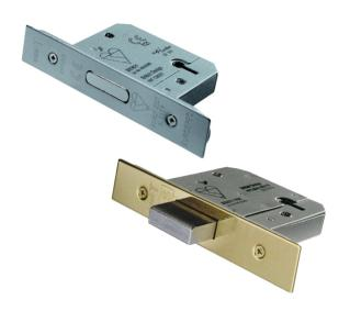
5 Lever BS Deadlock in 64mm and 76mm options. British Standard BS3621 Rated Dead Lock used as a matter of course by the national house builders. This lock provides a high degree of security and carries a 25 year mechanical guarantee. It has been CE and Certifire tested.
