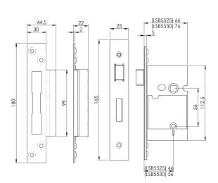
5 Lever BS Sashlock 64mm. The Latchbolt has the Easi-T reverse function to save undoing the case so it can be reversed in seconds. British Standard BS3621 Rated Sashlock used as a matter of course by the national house builders. This lock provides a high degree of security and carries a 25 year mechanical guarantee.
