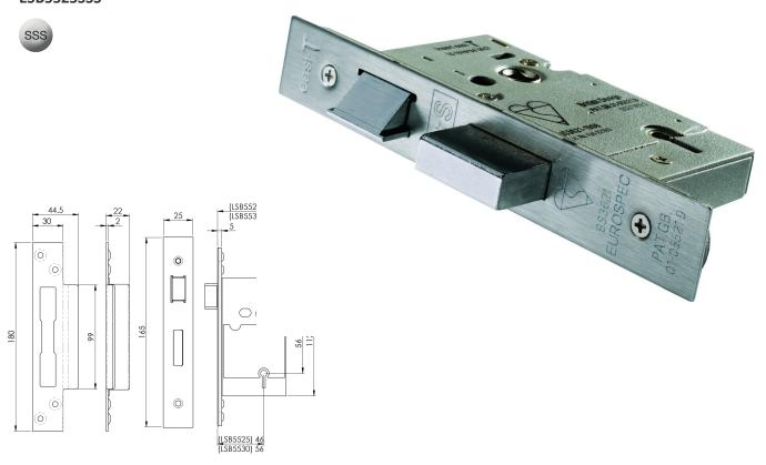
5 Lever BS Sashlock 64mm. The Latchbolt has the Easi-T reverse function to save undoing the case so it can be reversed in seconds. British Standard BS3621 Rated Sashlock used as a matter of course by the national house builders. This lock provides a high degree of security and carries a 25 year mechanical guarantee.
