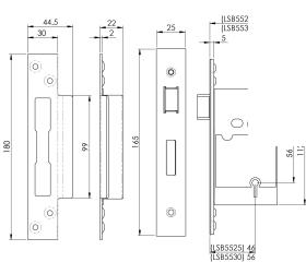
5 Lever BS Sashlock 64mm. The Latchbolt has the Easi-T reverse function to save undoing the case so it can be reversed in seconds. British Standard BS3621 Rated Sashlock used as a matter of course by the national house builders. This lock provides a high degree of security and carries a 25 year mechanical guarantee.
