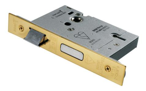
5 Lever BS Sashlock 76mm. The Latchbolt has the Easi-T reverse function to save undoing the case so it can be reversed in seconds. British Standard BS3621 Rated Sashlock used as a matter of course by the national house builders. This lock provides a high degree of security and carries a 25 year mechanical guarantee.
