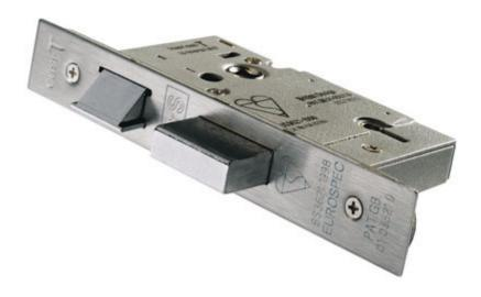
5 Lever BS Sashlock 76mm. The Latchbolt has the Easi-T reverse function to save undoing the case so it can be reversed in seconds. British Standard BS3621 Rated Sashlock used as a matter of course by the national house builders. This lock provides a high degree of security and carries a 25 year mechanical guarantee.
