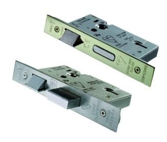
5 Lever BS Sashlock with 64mm or 76mm options. The Latchbolt has the Easi-T reverse function to save undoing the case so it can be reversed in seconds. British Standard BS3621 Rated Sashlock used as a matter of course by the national house builders. This lock provides a high degree of security and carries a 25 year mechanical guarantee.
