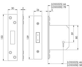
Easi-T Lever 3 Lever Deadlock in 64mm or 76mm options . Certified to BS EN 12209 Lock used as a matter of course by the national house builders. This lock provides a good degree of security and carries a 10 year mechanical guarantee. It has been CE and Certifire tested.
