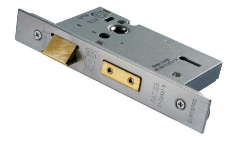
3 and 5 Lever Sashlocks. Square or Radius Forend versions with 64mm or 76mm options. The Latchbolt has the Easi-T reverse function to save undoing the case so it can be reversed in seconds. Certified to BS EN 12209 Lock used as a matter of course by the national house builders.
