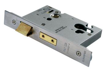
Euro Profile Sashlock in 64mm or 76mm option. The Latchbolt has the Easi-T reverse function to save undoing the case so it can be reversed in seconds. Certified to BS EN 12209. Used as a matter of course by the national house builders.
