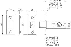
Tubular Deadbolt. with either 5mm or 8mm follower option. Commonly used as a bathroom deadbolt using a separate turn and release. Certified to BS EN 12209.
