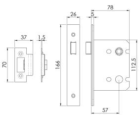
Upright Latch in 64mm or 76mm options. The Latchbolt has the Easi-T reverse function to save undoing the case so it can be reversed in seconds. Certified to BS EN 12209. Used as a matter of course by the national house builders.
