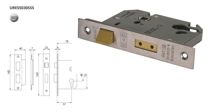
Universal Replacement Euro Profile Sashlock. 76mm. The Latchbolt has the Easi-T reverse function to save undoing the case so it can be reversed in seconds. Certified to BS EN 12209.
