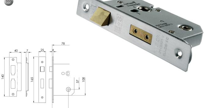
Universal Replacement bathroom Sashlock. 76mm. The Latchbolt has the Easi-T reverse function to save undoing the case so it can be reversed in seconds. Certified to BS EN 12209.
