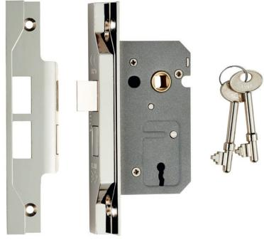
Contract 2 Lever Sashlock Rebated version 64mm. which comes with a pre-rebated faceplate and strikeplate for ease of fitting to pairs of rebated timber doors. The Latchbolt has the Easi-T reverse function to save undoing the case so it can be reversed in seconds. Certified to BS EN 12209.
