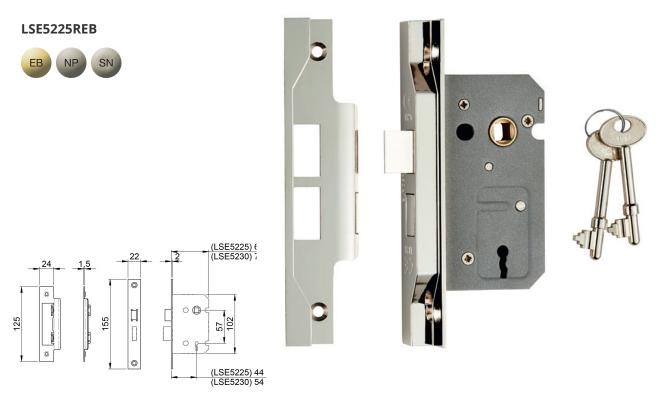
Contract 2 Lever Sashlock Rebated version 64mm. which comes with a pre-rebated faceplate and strikeplate for ease of fitting to pairs of rebated timber doors. The Latchbolt has the Easi-T reverse function to save undoing the case so it can be reversed in seconds. Certified to BS EN 12209.
