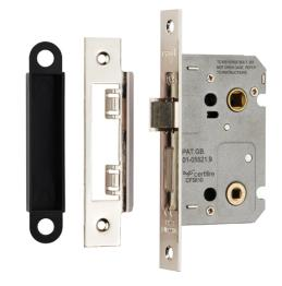
Contract Bathroom Lock, Square Forend. 65mm. The Latch bolt has the Easi-T reverse function to save undoing the case so it can be reversed in seconds. Certified to BS EN 12209.
