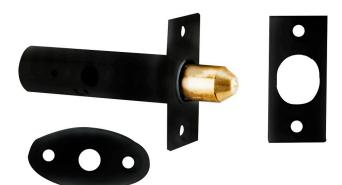
Contract Window Security Bolt, sometimes called a Rack Bolt. The bolt is morticed inside the window and can be locked or unlocked via a separate splined key or with a fixed splined turn. The bolt has an internal sawtooth rack mechanism into which the splined key is inserted. The spline engages with the rack teeth and forms a gearing action which smoothly operates the bolt.
