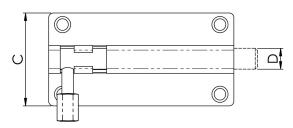
Standard straight barrel bolt. The simple and popular basic door security device. The bolt is slid into the staple and the finger knob is rotated to engage in the housing slot thus locking it in position. Architectural quality.
