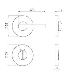
Thumbturn and Release on a concealed fix press on rose. The turn side has a long straight tubular bar, and the release side has a vacant/engaged indicator. Ideal for public/office toilet doors where a more ergonomic operation is a necessary requirement. Part of the Steelworx range in G201 Stainless Steel.
