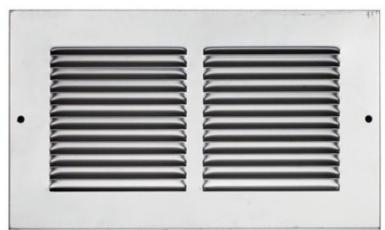
Face plate cover for ES air transfer vent ES404 designed for use in fire resisting doorsets and compartment walls. When dormant, the grilles allow air to circulate throughout the building. In the event of a fire they are designed to close and restrict the flow of hot gasses and fire. All air transfer grille systems are tested to BS476 part 20/part22:1987 - 30 and 60 minute fire rated.
